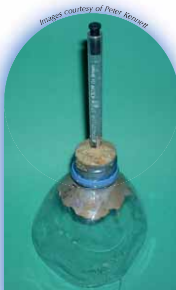
Home-made funnel using the top of a bottle, a tube from a ball-point pen and some clay
